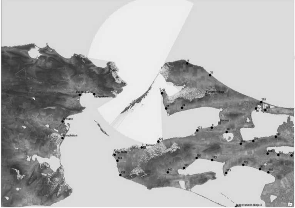
Fig. 10. Visibility study from Ilich into the Kerch Straits and adjacent areas. Viewpoint is 20 m above surface level, the visible zones are represented in light grey. Based on SRTM 30 data, calculated with ARCGIS (© D. Kelterbaum)
